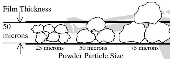
Packed, uniform spheres result in void spaces of upto 48%. Thermosetting powders however consist of irregular multi-sided particles of varying size and psd. When these powder particles are deposited in a layer the void volume will be greater. Therefore, before melting and cross-linking the powder film can be between three and seven times the actual thickness of the final coating film after curing.
