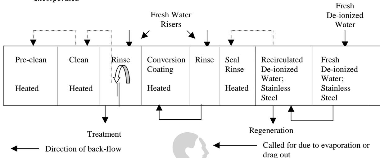
**Conversion Coating** - Once all impurities on the metal surface have been removed the surface is ready to be conditioned for optimal adhesion of the coating film.
