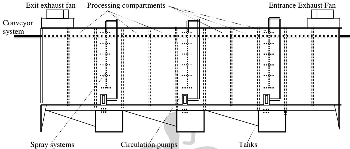
Figure 7: Examples of Spray Risers
